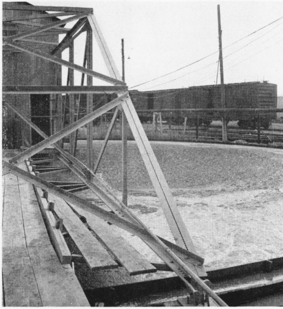
After being dug out of the earth the ore is heated to a high temperature in a concentrator like this as part of the refining process. While the ore is going through the refining process it is commonly known as "spelter."
